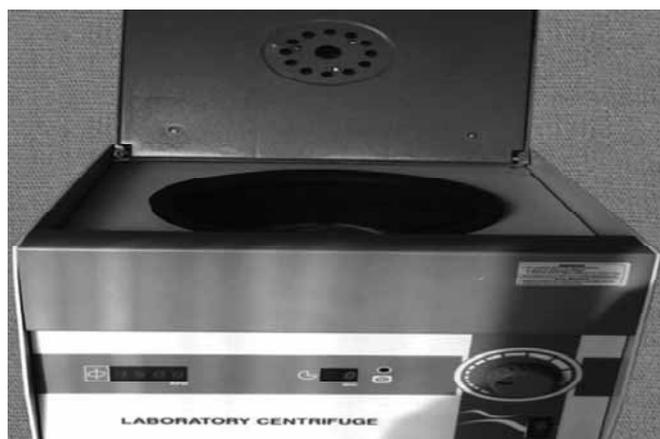
Fig. 1: Digital centrifugal machine
