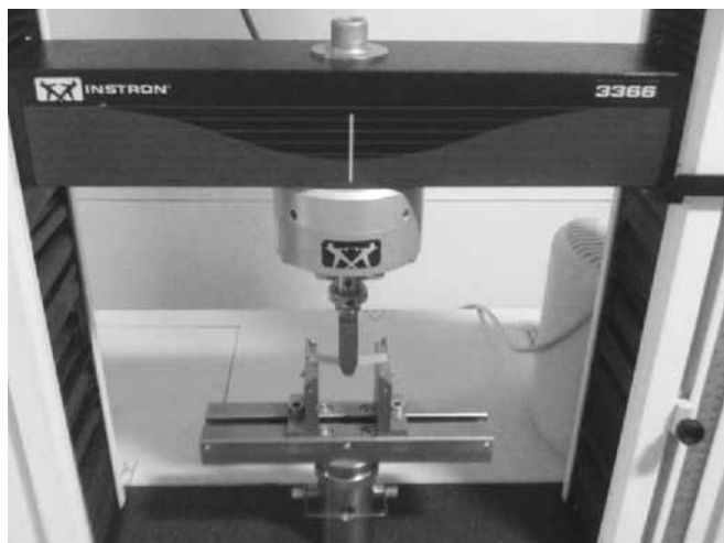
Fig. 1: Measurement of flexural strength using Instron
