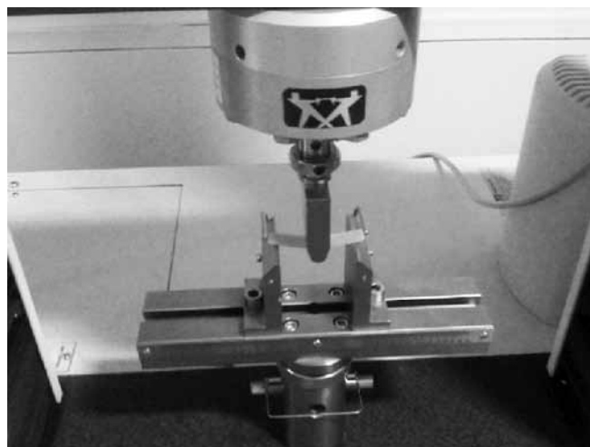
Fig. 1: Measurement of flexural strength using Instron
