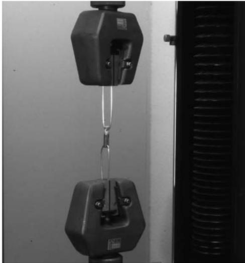
Fig. 5: Casting being tensile tested on universal testing machine
