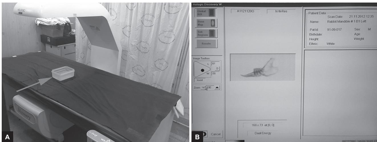
**Figs 1A and B:** Hologic WI bone densitometer device. A semi-mandible was sunk in the cubic thin-walled plastic filled with water up to a height of 8 cm and the device was set for starting the test: (A) The red arrow shows position of the plastic container, (B) the device setting applied on software before starting the test
