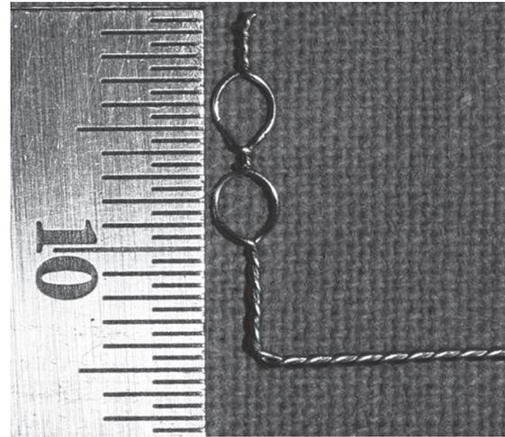
**Fig. 1:** Implant guide design with 2 mm gap between the loops
