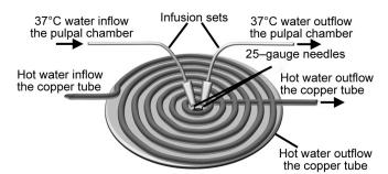
**Fig. 2:** Bottom view of the temperature-controlled aluminum base plate (TCAP), which is part of the experimental apparatus to regulate the tooth physiological temperature
