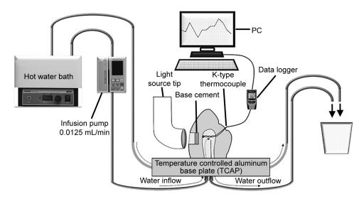
Fig. 1: Schematic drawing of the mandibular premolar tooth and class V cavity with experimental microcirculation apparatus
