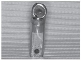
Fig. 4: Cemented and vented casting prepared for testing
