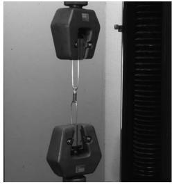
Fig. 5: Casting being tensile tested on universal testing machine
